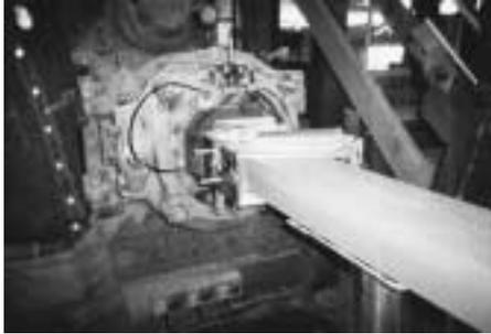
**A slab of clay emerges from the extrusion machine before being sliced into bricks**
