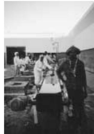
**Bricks are scrubbed clean manually to remove the coal ash stains**
