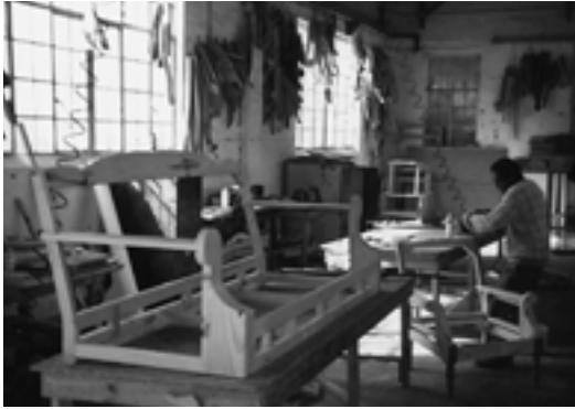
Cutting and assembling frames in the frame shop
