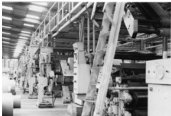
*Transformation machine processing cardboard into finished product*
